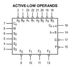
V<sub>CC</sub> = PIN 24 GND = PIN 12
